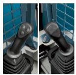
Easy-to-operate Control Levers Short-stroke hydoraulic pilot control levers provide precise, vibration-free operation with less fatique. H-pattern and ISO-pattern joysticks are available as options.
