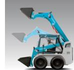
Self-leveling System Simply by operating the lift pedal, the bucket stays even and level when the arms are raised.
