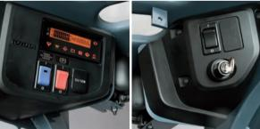
The instrument panel comprises separate left and right sections, for outstanding upward visibility. The layout of the front and rear pillars is nearly parallel, providing a spacious operator compartment.
