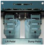
Rugged Lift and Dump Pedals The pedals are shaped to minimize slips, even with muddy boots. They control hydraulic lift and dump, and the bucket can be "floated" by toeing the lift pedal into a detent position.
