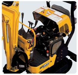
Fully openable hood for easy maintenance and detachable side cover
